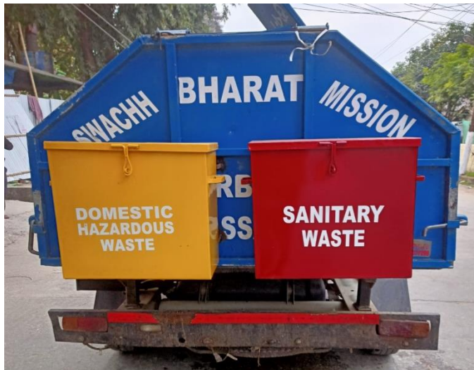
D2D Vehicle retrofitted
